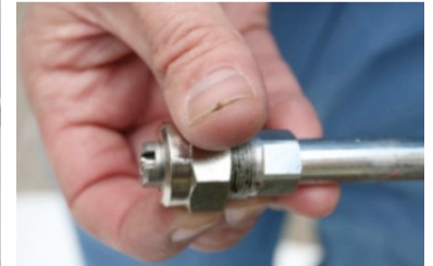
Image 3: Attach the spray-tip.
