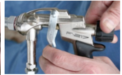
Image 4: Black valve to adjust spray pattern.
