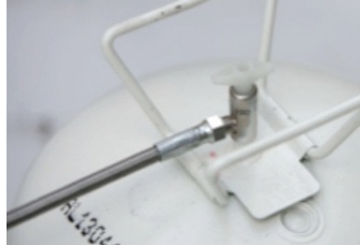
Image 1: Canister with the braided-hose attached properly.
